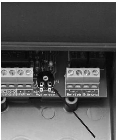
Fig. 4: Setting the differential gap
