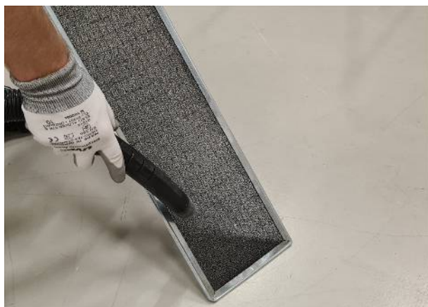
Fig. 25: Vacuum the filter and re-fit it after cleaning.
